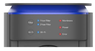
Figure 1. Smart RO unit LED indicators
